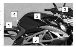
Loose hex socket bolts M6 on shifting arm and on shifting lever for remove quickshifter sensor from motorcycle.
